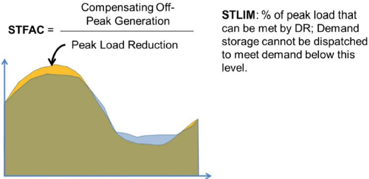
Fig. 2. Illustration of key DR parameters in GT-NEMS.
