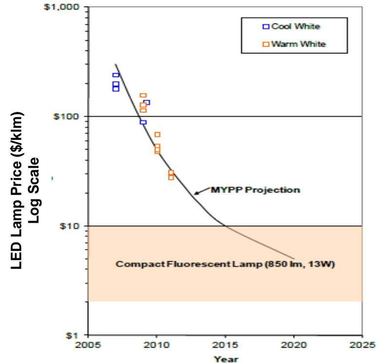
[Figure] White Light Integrated LED Lamp Price Projection (Logarithmic Scale)
