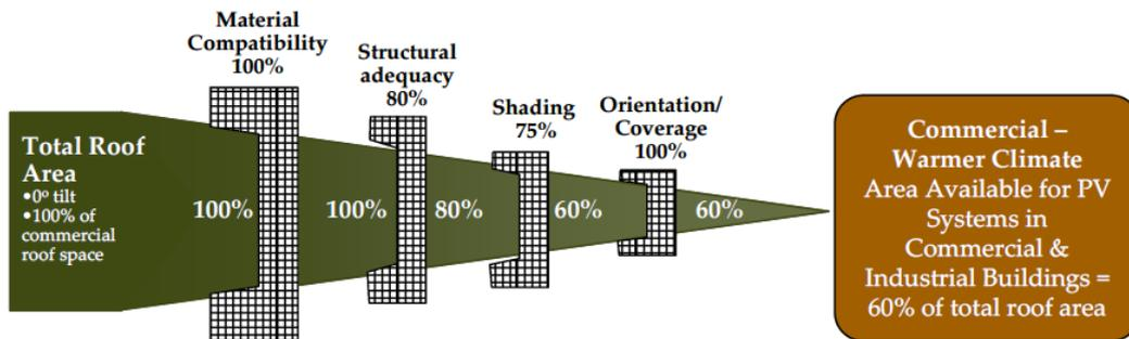
60%-65% of the commercial rooftop area is suitable for solar PV installation.
