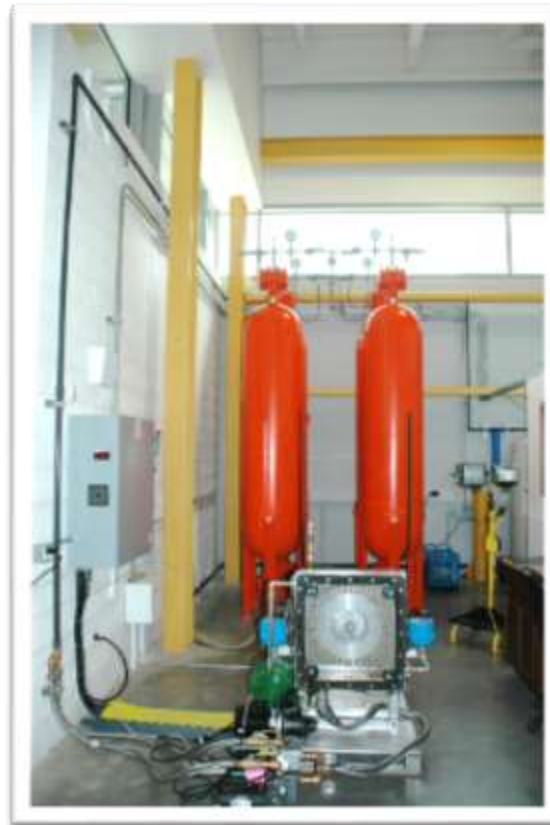
GLIDES first- generation proof-of- concept prototype
