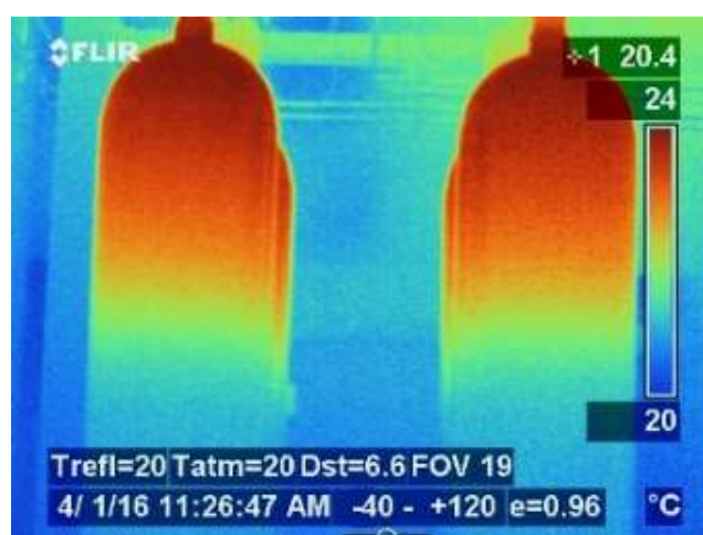
Infrared thermal image of GLIDES prototype storage vessels during charging
