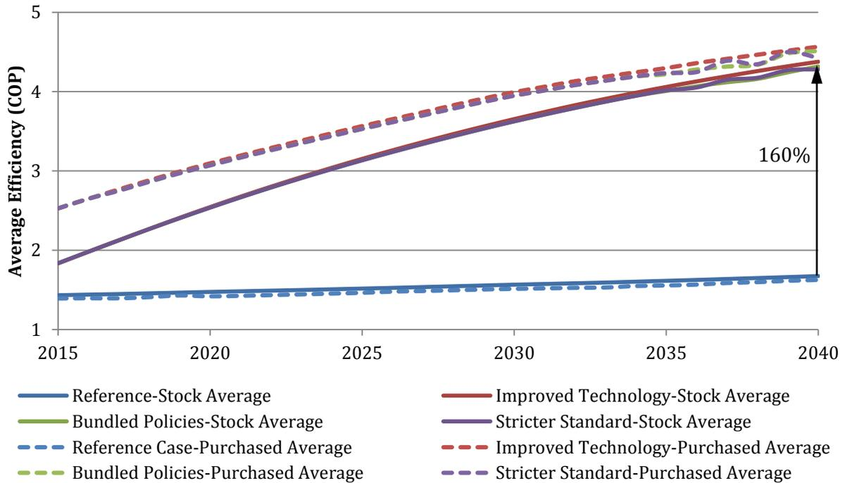
**Figure 6. Improved Efficiency of Electric Space Heating**
